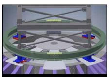
The Brock EVERLOC® Mount provides a strong and flexible base for the bin peak support tower. The mount system's ring component allows for flexibility if changes are needed in the future. Bolt-together assembly can be installed during bin construction and can also be adjusted to ensure the position of the support tower easily aligns to the equipment being attached.
