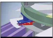
Weather-Tight - From the top side this is a clean connection. All assembly is a bolt-together design, minimizing the size of openings needed in the roof skin. As with the underside components, the mount system assembly can be accomplished while the bin is being constructed closer to ground level.
