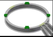
**Starting Point** - Where the attachments are made directly to the compression ring under the roof skin.
