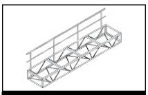
**Bottom Box Truss** comes in standard widths of 27-60 inches (686-1524 mm) and maximum span of 55 feet (16 m).
