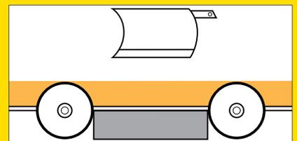
STEP 3: To return to by-pass operation, the discharge moldboard raises while the belt support frame lowers allowing the belt to return to its normal conveying profile.
