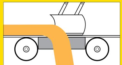
STEP 2: In discharge operation, synchronized actuators raise belt support frame to flatten belt profile, and the curved discharge moldboard plow lowers into contact with conveyor belt to divert material and fines.
