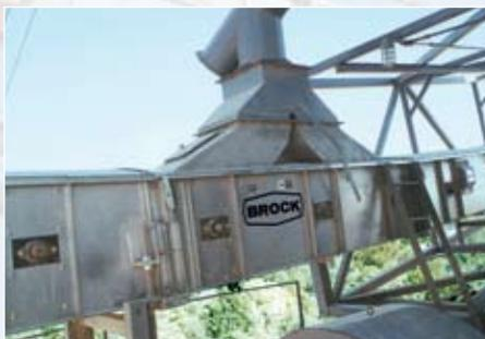
2-way inlet for Brock's reversing conveyor configuration
