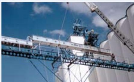
Pre-assembled and shipped in sections up to 40 feet (12 meters)
