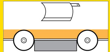
STEP 1: In by-pass operation, material flows through to the end of the conveyor.
